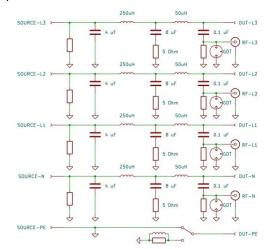
Figure 2 – 3-phase LISN, simplified schematic
