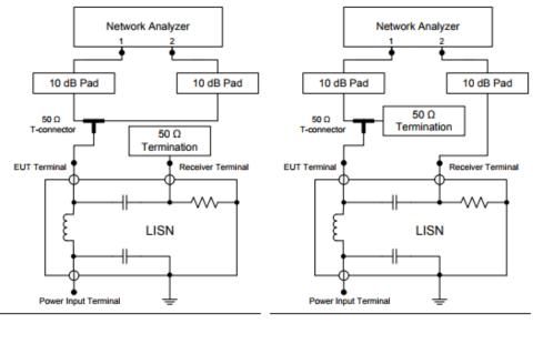
Reference measurement setup using network analyzer. Transmission measurement setup using network analyzer.
