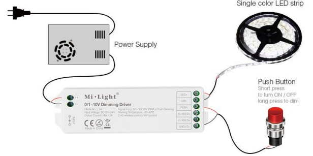
Push button connection diagram
