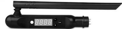
Each DMX light bulb / strip controller or each group of DMX light bulbs / strip controllers use 5 DMX 512 communication channels, those 5 channels can adjust the brightness of red, green, blue, warm white, cool white, from 0% to 100%.
