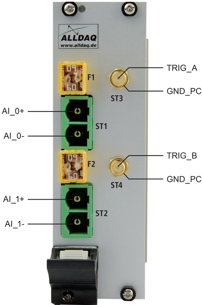
Figure 9: Connectors of the ADQ-412
