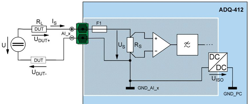
Figure 5: Wiring the current measurement channels
