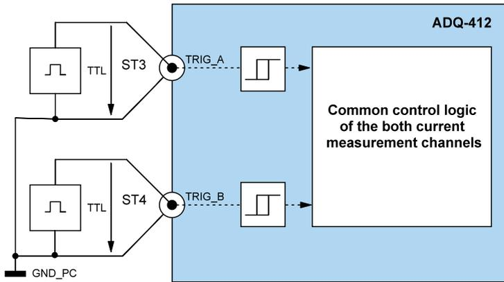
Figure 6: Wiring of the external trigger inputs
