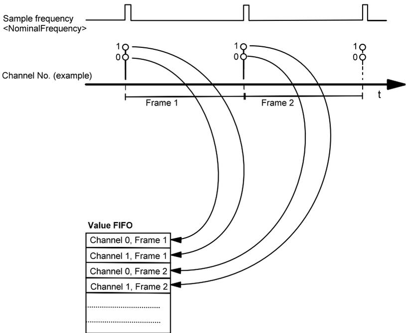
Figure 7: Timer-controlled acquisition
