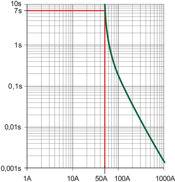
Figure 8: Characteristic of the fuse
