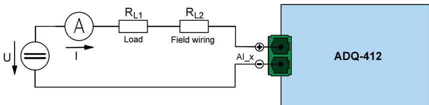
Figure 2: Wiring for adjustment
