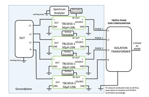
Picture 16: Measurement set up for triple phase AC supplied equipment in Star configuration
