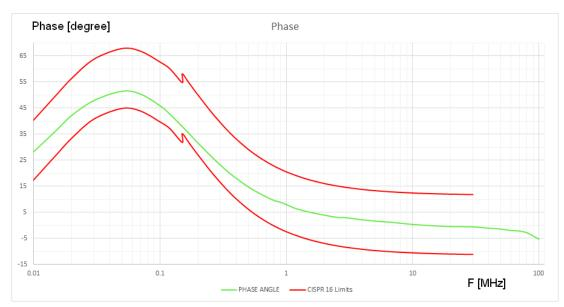
Picture 3: LISN phase,  $50\Omega$  //  $50\mu$ H +  $5\Omega$
