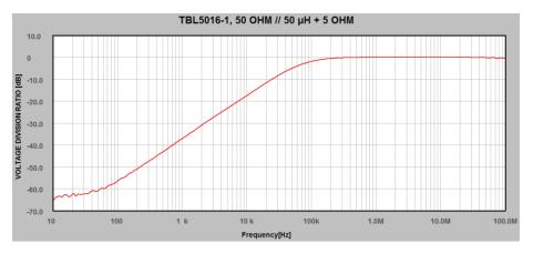
Picture 8: Voltage division ratio DUT terminals to RF connector,  $50\Omega // 50\mu H + 5\Omega$
