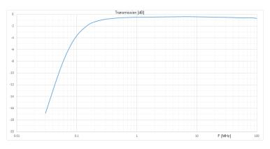
Picture 11: Transmission , DUT terminals to RF connector,  $50\Omega\,/\!/\,50\mu H$
