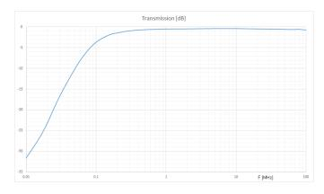
Picture 10: Transmission , DUT terminals to RF connector,  $50\Omega\,/\!/\,50\mu H$  +  $5\Omega$
