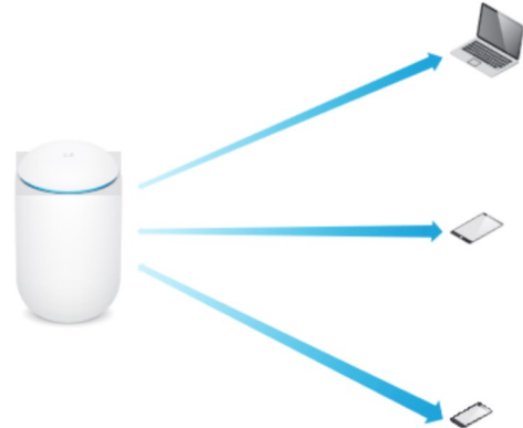
MU-MIMO with 2x2 and 1x1 clients: The UDM communicates with one 2x2 client and two 1x1 clients at a time.
