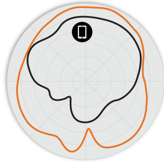
Figure 3. H550 5GHz Azimuth Antenna Patterns
