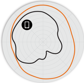
Figure 2. H550 2.4GHz Azimuth Antenna Patterns
