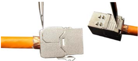
⑩.Press down the retainer for 360 degree shielding
