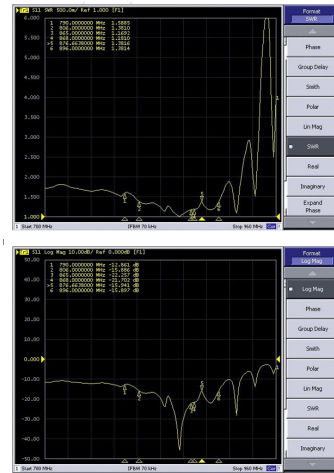
VSWR and Return Loss Model: ANT-868-14dbi-Yagi 14 Elements
