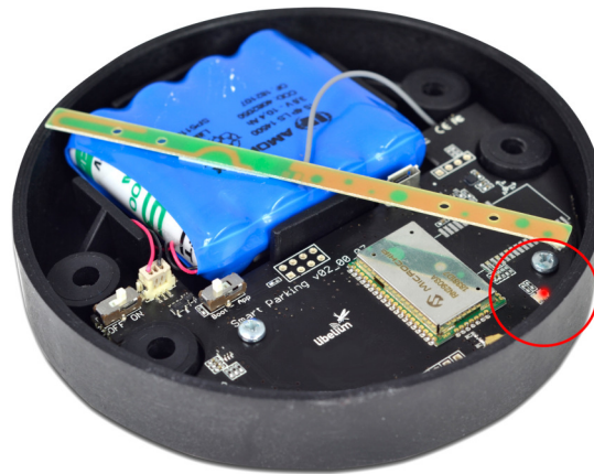
Figure : The red LED blinks once to indicate ready-to-install state
