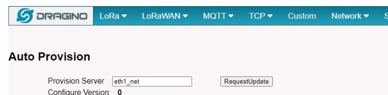
The screenshot shows the DRAGINO web interface with the "Auto Provision" section. It includes fields for "Provision Server" (set to "eth1\_net") and "RequestUpdate", and a "Configure Version" field set to "0".
