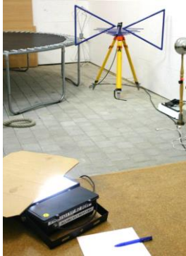
Radiated emissions measurement at 100W (max hold)
