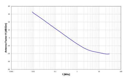
Figure 1: magnetic field antenna factor, TBMA6-P, 60 cm loop, 9 kHz - 30 MHz, typical data
