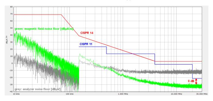
The above screenshot shows the magnetic field noise floor of a set up consisting of a low-cost spectrum analyzer and the TBMA6-P loop antenna.
