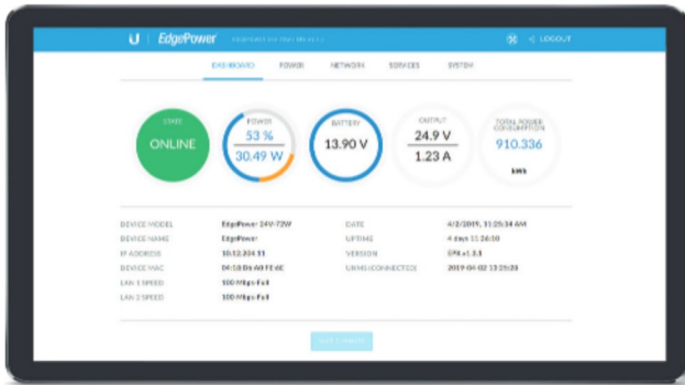
Use the local web UI to monitor and configure the EdgePower
